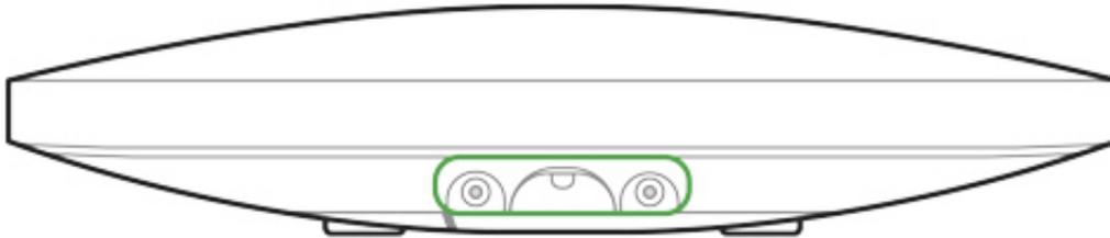
Do not flip the range extender when attaching vertically (for instance, on a wall). When properly fixed, the Ajax logo can be read horizontally.
