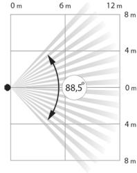
Horizontal and vertical viewing angles of the detector
